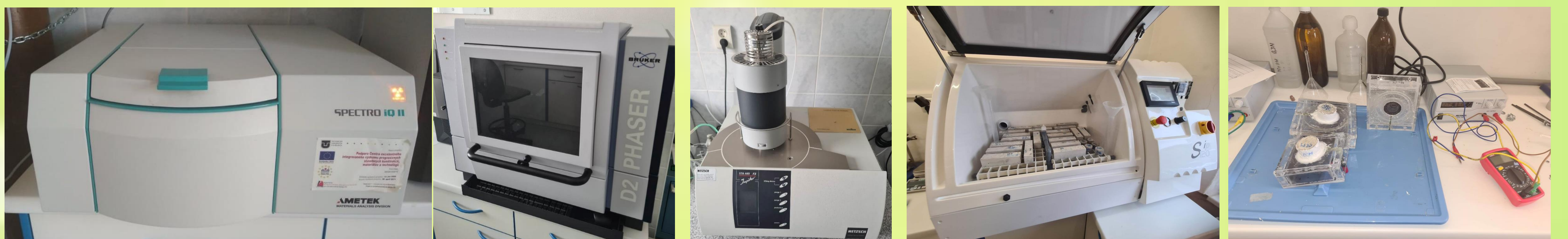
Figure 3: X-ray fluorescence spectrometry, X-ray diffraction analysis, Thermogravimetry-differential scanning calorimetry, Corrosion Chamber for acid rain simulation (1 year in real conditions), Rapid Chloride Permeability Test Apparatus for ion diffusion.
